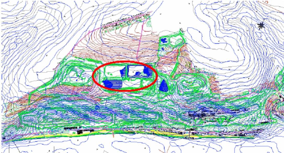
Figure 5. Superimposition of Elevation maps created from DTM and DEM and AutoCAD drawings The DTM map is in grey, the DEM map blue.
